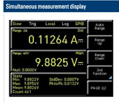
Simultaneous display of three measurements, including DCl and ACl at the same time.  $\label{eq:constraint}$
