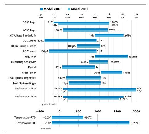
Both the 2001 and 2002 provide exceptional measurement range. In addition, the 2002 offers extended DCV and resistance measurement capabilities.
